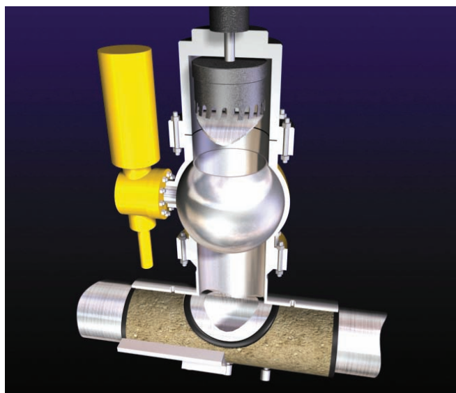
Hot tapping using Grouted Tee connection
